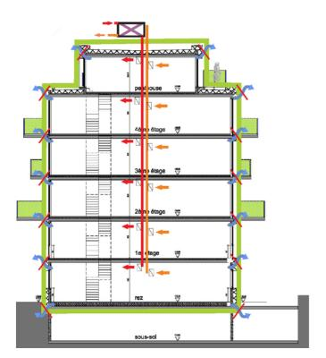
Insulation, airtightness and ventilation of the building
